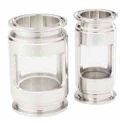
Inline tri-clamp, double window sight glass for media and purified water applications for the food & beverage and consumer health and beauty industries. Suitable for CIP and SIP, the SG Series has a large viewing area, full bore flow path, and a metal stop that provides ideal o-ring compression and prevents pipe torque from affecting glass.
