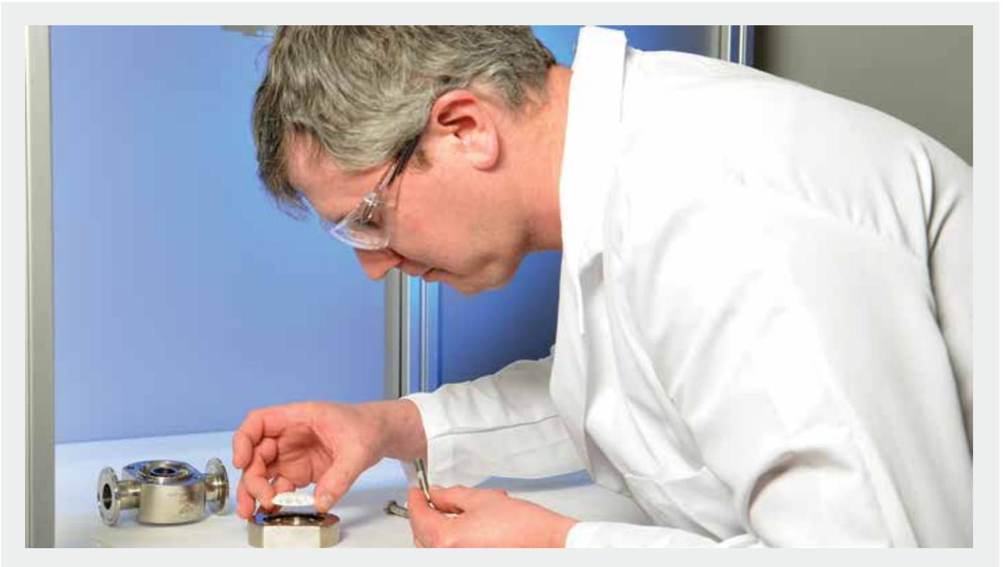
Biopharmaceutical process design engineers have rarely felt comfortable specifying "sanitary" spring check valves in WFI, buffer or direct process applications. The crevices, exposed springs, high particulate and cracking pressure with increasing differential pressure at increased flow, are just some of the reasons that spring and stem guided check valves are not used. Those are the specific reasons the SVC and SHC check valves were developed.
