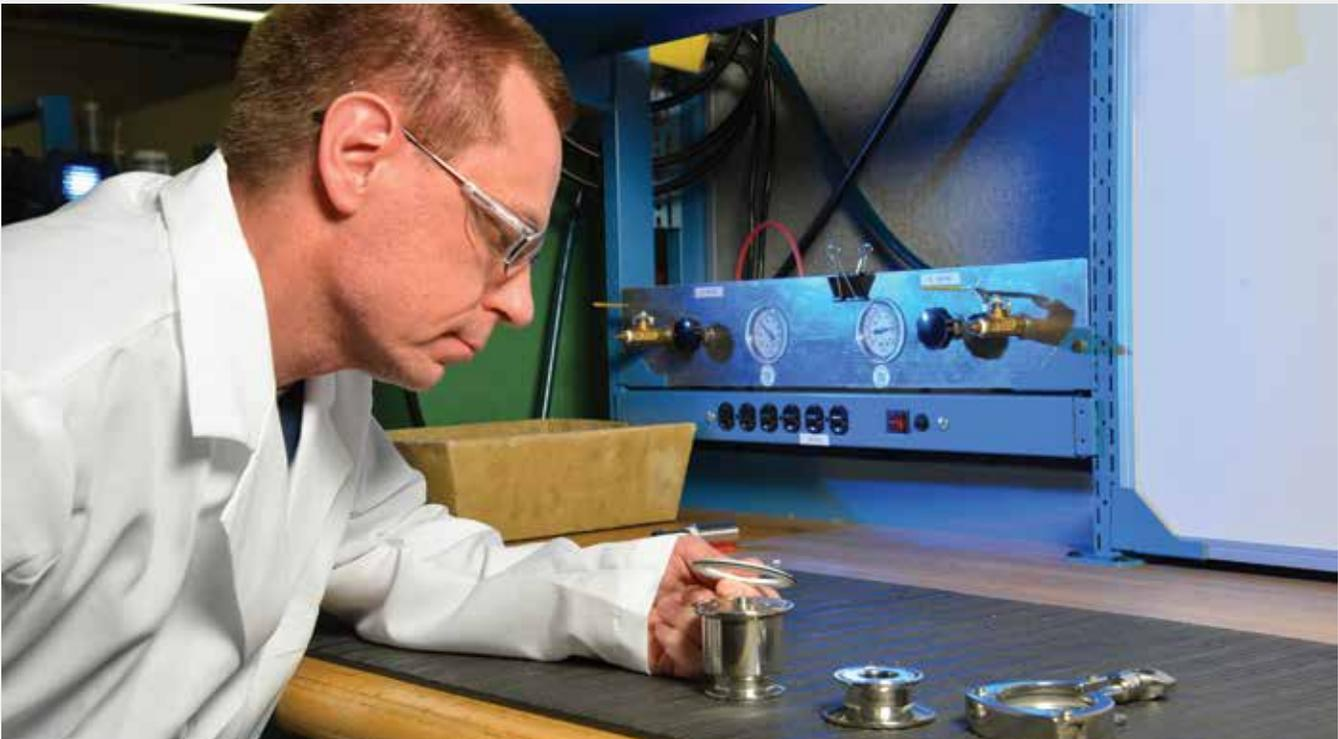
Biopharmaceutical process design and maintenance engineers know that the two most important criteria for choosing a clean steam trap for draining SIP condensate are low subcooling operating and maintenance reliability. Without either, you will have unexpected downtime caused by slow SIP heat-up or validation temperature sensor alarms.
