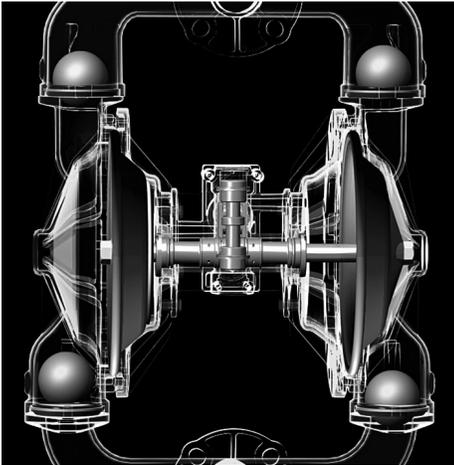
The air-valve directs pressurized air behind the diaphragm on the right, causing the diaphragm on the right to move outward (to the right).
