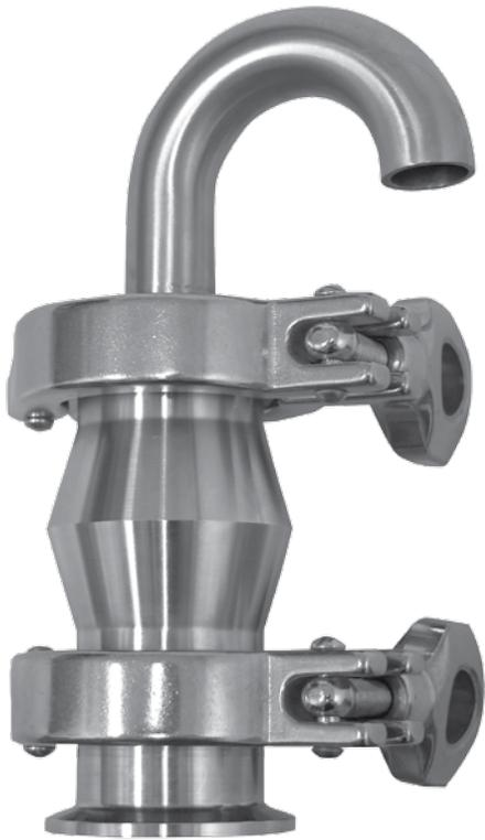
The TL60ARV Air Relief Valve is used primarily when removal of air from a line without loss of product is a concern. The design of the TL60ARV is simple: a ferrule, a housing with a plastic ball, and a vent pipe all connected using 2 standard heavy duty clamps. This design will not let air enter the line or container under negative pressure.
