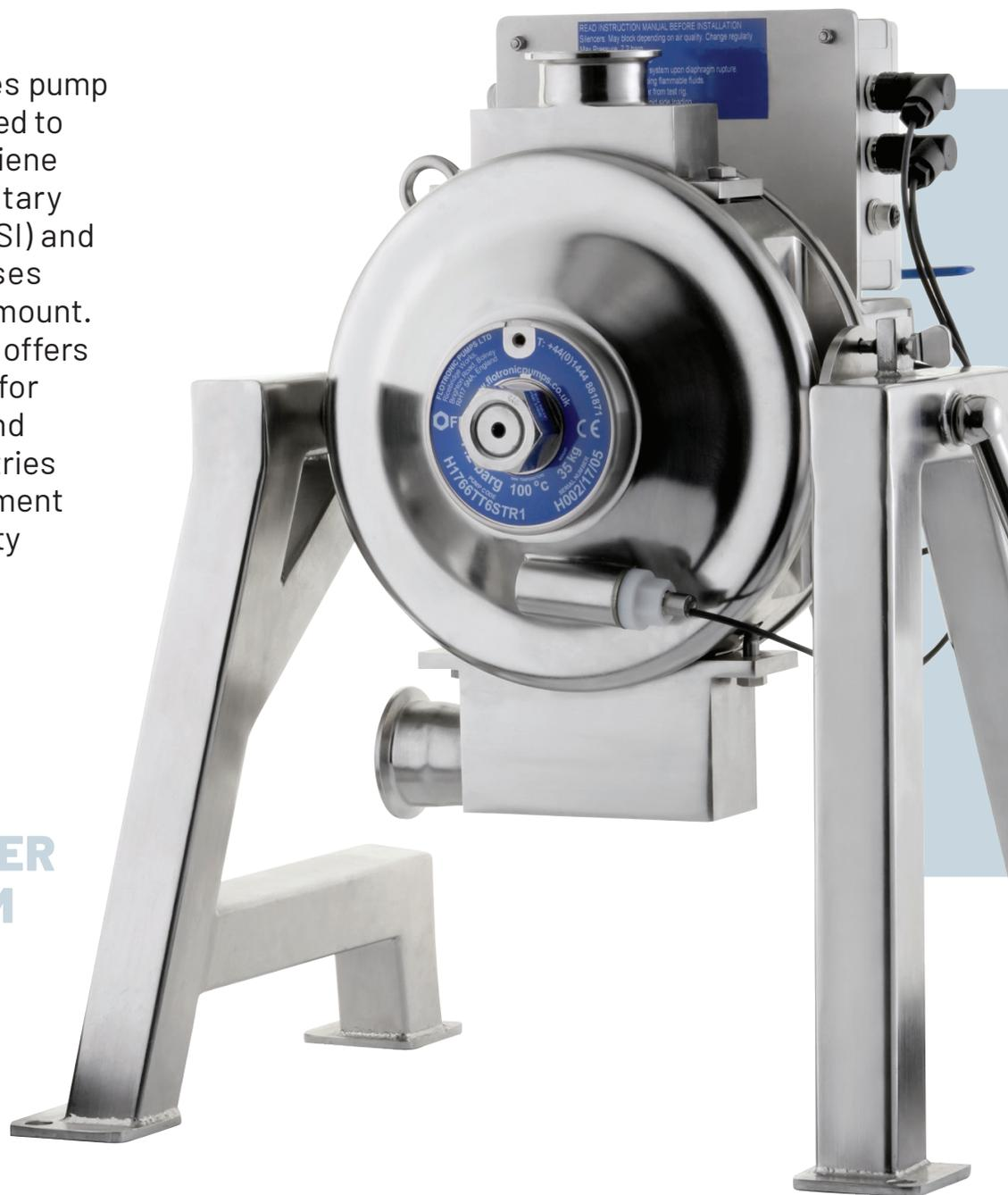
H-Series pump parts and raw materials are of the highest quality with their provenance duly certified. Product contact areas are either PTFE or 316L Stainless Steel, with stainless product contact areas polished to 32µin Ra maximum. Cleanability is further enhanced by an electro-polished overall finish.
