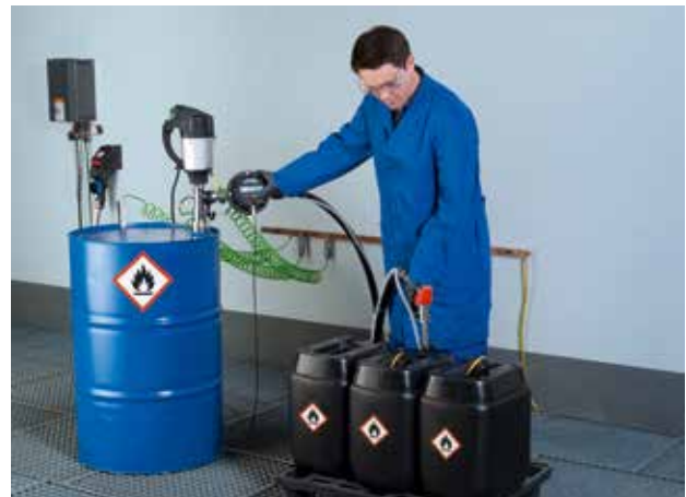
Semi-automatic can filling in explosion zone 1.
