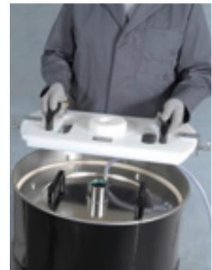
Assembly pump centring plate.\*
