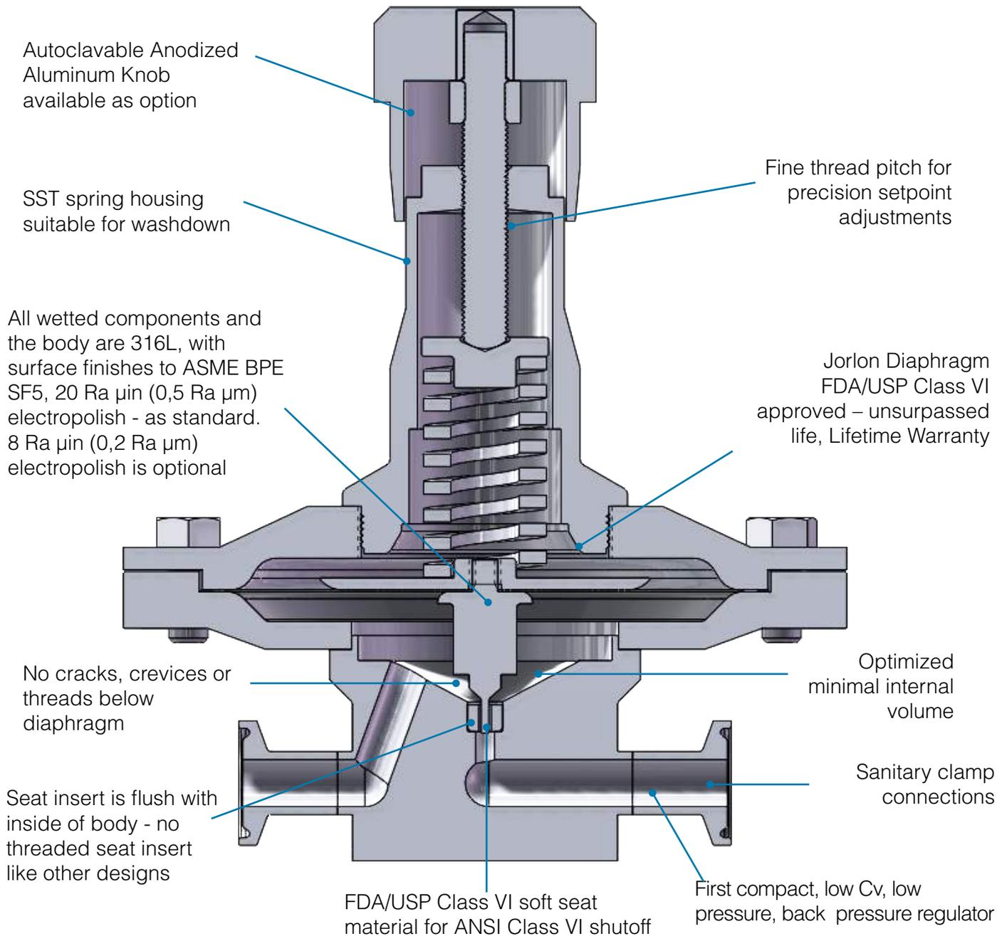
**Note:** The orifice for the JSBLFLP's unique soft seat is machined after insertion in the body during manufacturing. The seat insert cannot be replaced in the field. If repair parts are required, a spare body with insert is recommended, along with standard replacement parts of stem and diaphragm. After the body is replaced, it may be sent back to the factory for seat replacement.
