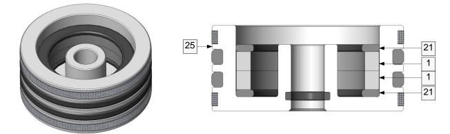
Place a first seal [21] inside the jack piston [25], then 2 ring magnets [1] and then a second seal [21].
