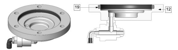
Install the seal [19] after greasing it in the jack base [12].
