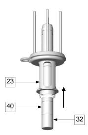
Place the PFA scraper seal [26] and the ring [27] on the piston rod [32] and fit the assembly using the specific tools [40] and [41] into the lantern [23].
