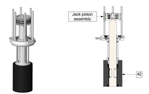
Use the retracted rod maintenance base [42] to lower the jack piston assembly to its lowest point.
