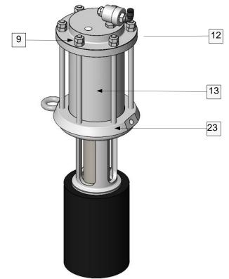
Finish fitting the jack barrel [13] with the jack base [12] into the lantern [23], tightening the greased double nuts [9].
