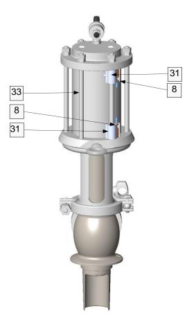
Assemble the detector holders [31] with the magnetic detectors [8] and attach them to the tie rods [33].
