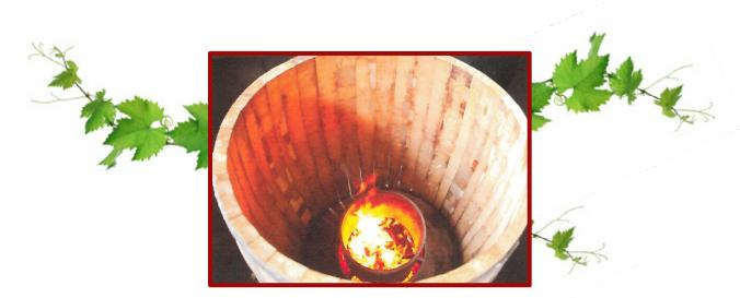
The toasting process is carried out under the watchful eye of a Master Cooper and is accompanied by careful sprinkling. Wood fibers, rendered flexible by the heat and humidity, can now be bent using a winch to gradually arch the staves and tighten them for obtaining the shape of the barrel.
