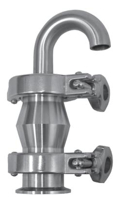
The TL60ARV Air Relief Valve is used primarily when removal of air from a line without loss of product is a concern. The design of the TL60ARV is simple: a ferrule, a housing with a plastic ball, and a vent pipe all connected using 2 standard heavy duty clamps. This design will not let air enter the line or container under negative pressure.
