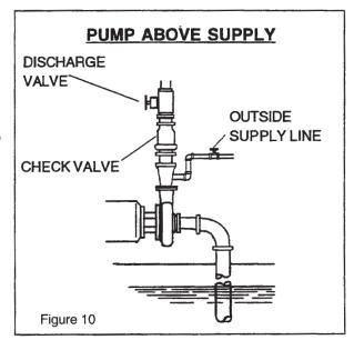
8. Slowly open the discharge valve until desired flow is obtained. Observe pressure gauges and if pressure is not attained quickly, stop pump and prime again.
