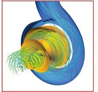
The helicoidal impeller is designed with the CFD tool (Computational Fluid Dynamics)
