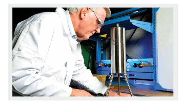
Steriflow's sample coolers are constructed to higher quality standards than others we have tried.... You can see the care taken with the exterior construction. But it's more than that. The single piece of uncut, unblemished sample tubing from sample inlet to outlet means less probability of sample contamination. It's that simple.
