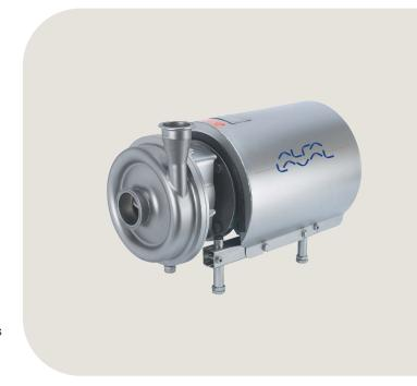
A compression coupling securely attaches the stub shaft to the motor shaft with precision alignment, and the semi-open impeller with a special vane design ensures efficient and gentle handling of the product as it moves through the pump.
