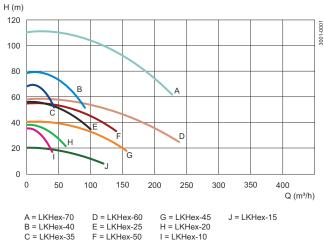
Frequency 50 Hz, Speed (Synchr): 3000 rpm
